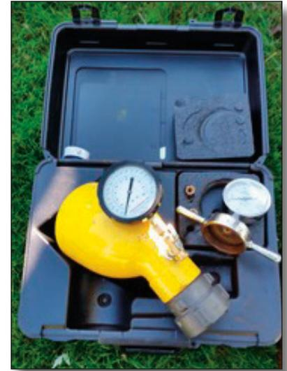
the Internet. Plug in the numbers and print the results. NFPA recommends flow testing of underground and exposed piping at least once every 5 years (NFPA 25, Table 7.1.1.2, 2014).
