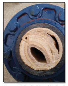
is slightly alkaline causing issues with the leeching of lead and copper. The DOH confirmed that this was the case. Elevated lead and copper levels resulted in the requirement to adjust the pH and to add a layer of protection that the caustic soda provides.
