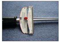
Beam-type torque wrench. The indicator bar remains straight while the main shaft bends proportionally to the force applied at the handle.
